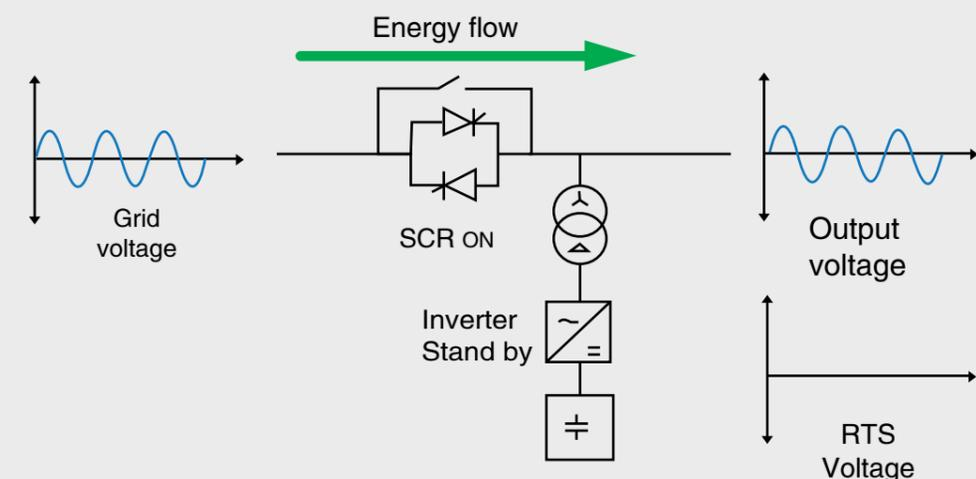
When voltage sag occurs, AVC-RTS immediately controls the thyristor to turn off, and the grid voltage is completely isolated from the load. Within 5ms, after being discharged by the inverter, a preset voltage is output to the load through an injection transformer. The voltage support of AVC-RTS completely avoids the harm to the load caused by voltage sag.
