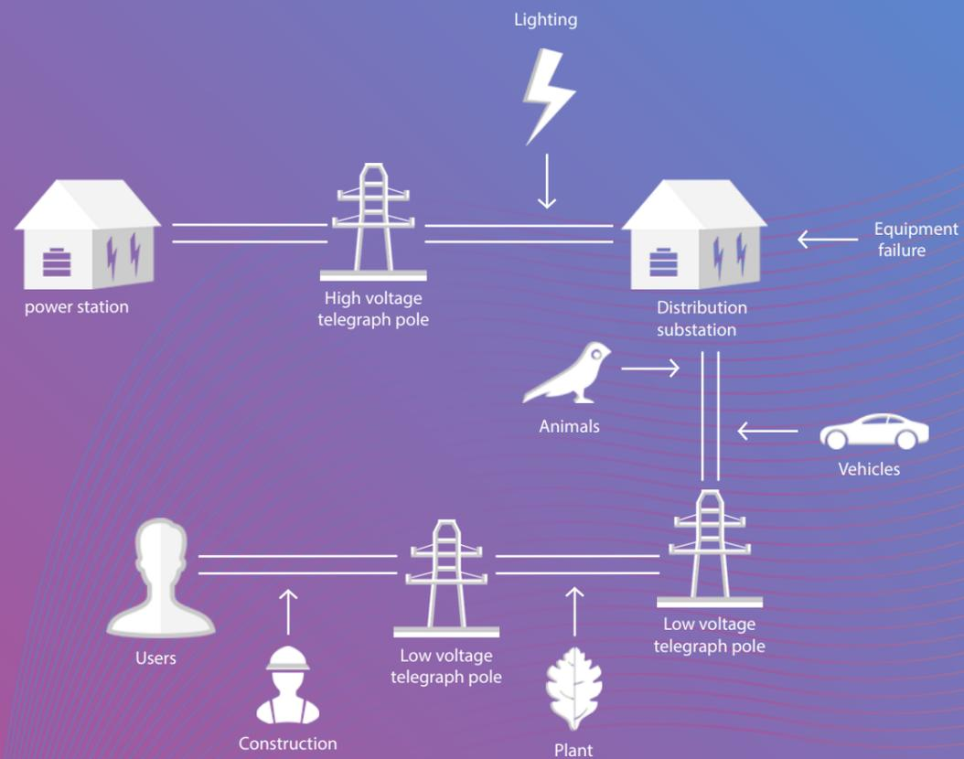
Voltage sag is generally caused by the failure of power grid, substation facilities or sudden large changes in load. In the process of long-distance transmission, there are many unpredictable situations, such as power system fault, lightning strike, large motor starts, capacitor switching and other events in the transmission and distribution system.
