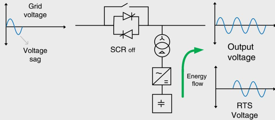
When the grid voltage returns to normal value, AVC-RTS stops working and controls the thyristor to turn on, the output voltage returns to the grid voltage, and the super capacitor begins to charge in preparation for the next voltage sag.
