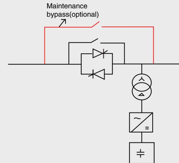
When the grid voltage is within the normal range, AVC-RTS standby, the control thyristor turn on, the inverter is not working, and the super capacitor is in full power state. The output voltage is the grid voltage.
