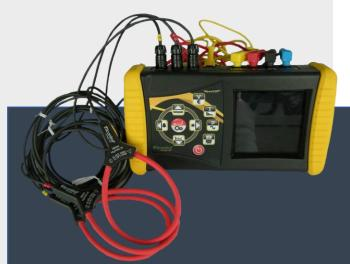
NANOVIP® CUBE™ is a modern, powerful, portable network analyzer developed for professional analysis of consumption and power quality of the most complex electrical networks.
