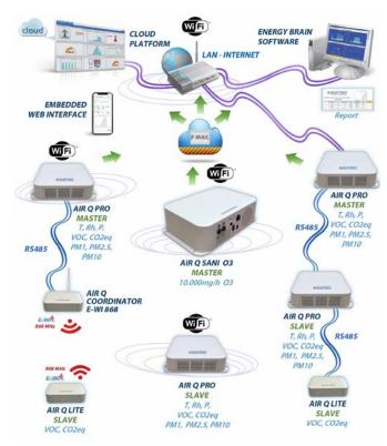
In the example there is an AirQ SANI <sup>O3</sup> that implements the sanitation of the rooms and is networked with other AirQPro and AirQLite devices inserted in different rooms for monitoring the local air quality. The devices are connected to each other both via Wi-Fi and Ethernet cable but also using a 868MHz radio communication via the Deca Coordinator E-Wi 868. For further information on Electrex networks and their advanced and innovative functions, refer to the website www.electrex.it.
