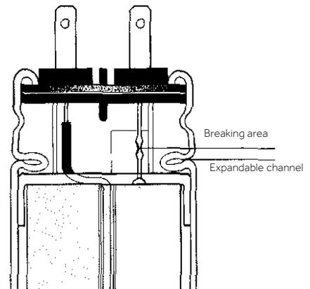
The formation of electric arcs inside is prevented by the presence of **insulating oil**, of vegetable type, which immediately penetrates the breaking point of the wires.
