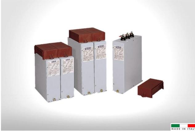
The three-phase modular capacitors of the **CT** series, available in three types, are designed for low-voltage power factor correction. The construction of the capacitors is made to guarantee excellent thermal dissipation. Three single-phase units are assembled inside, each equipped with an anti-burst device.
